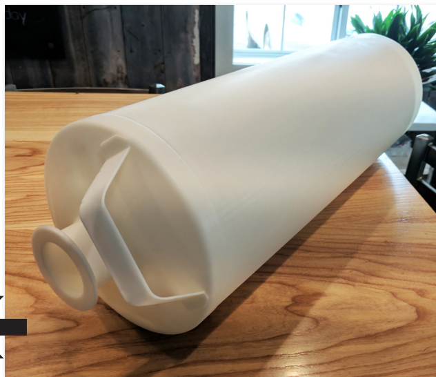
The supports built with the canister and lid during the 3D printing process were removed, and the canister and lid were assembled to check for accuracy.
