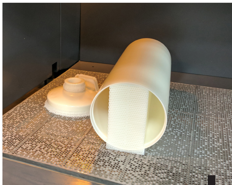
A 3D scan of the canister was input into the UnionTech RSPro 800, then the canister and lid were built separately on the platform of the printer at RP America's 3D printing lab.
